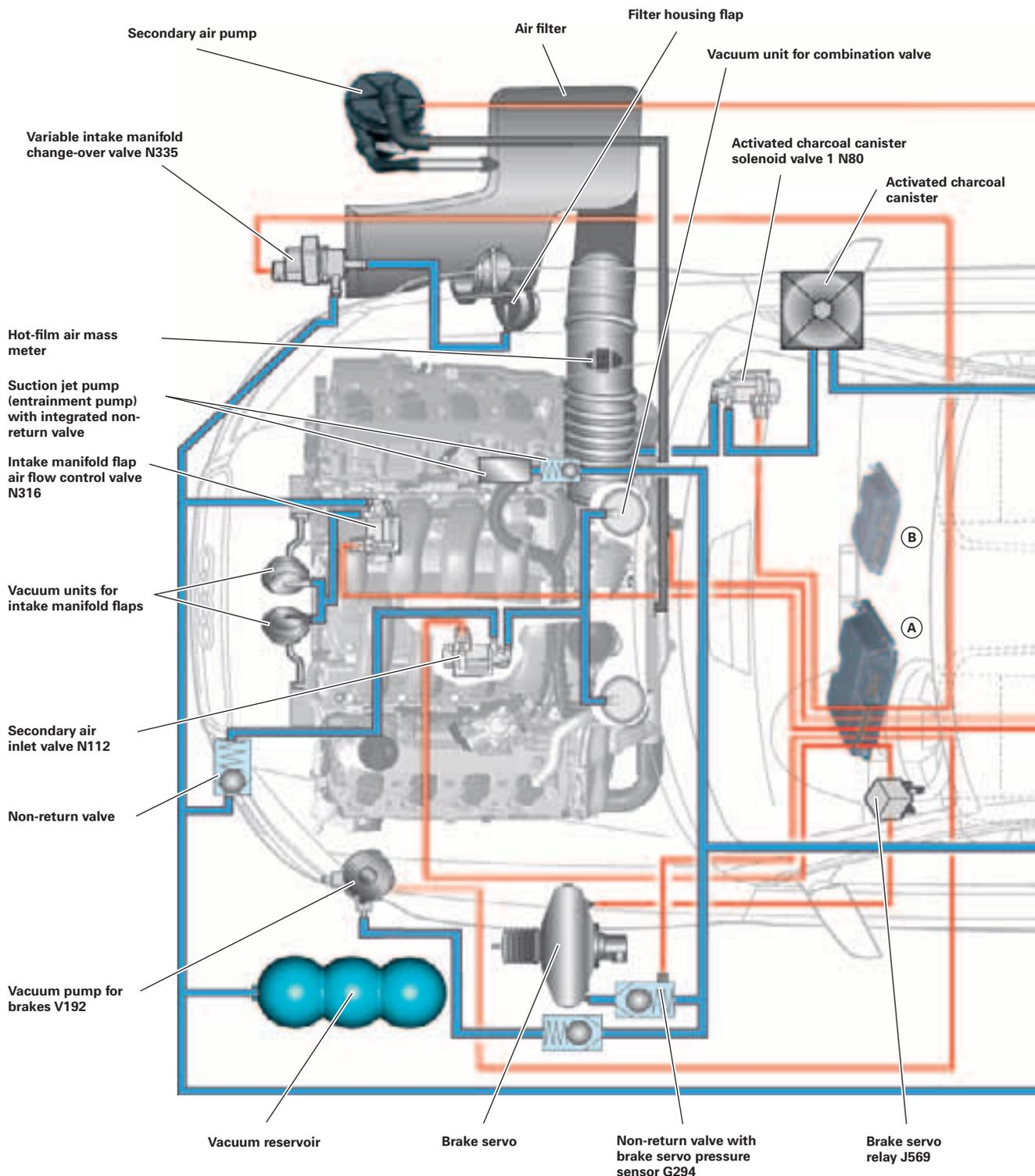
For this reason, in both engine versions, the requisite vacuum is produced by a suction jet pump and, if necessary, additionally by an electrical vacuum pump.
