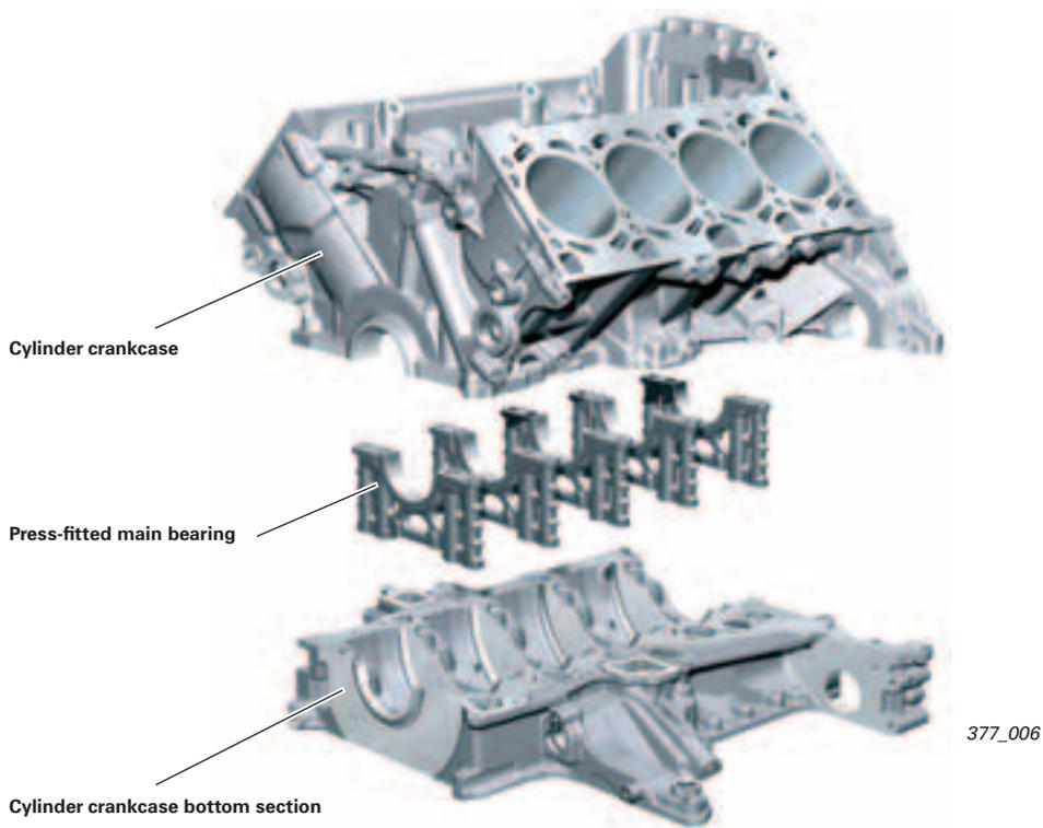
The **cylinder crankcase lower section** (bedplate bearing cross-member) is made of aluminium with press-fitted iron main bearing covers made of grade 50 nodular cast iron. It is centred using centring pins, sealed with liquid sealant and bolted to the cylinder crankcase.
