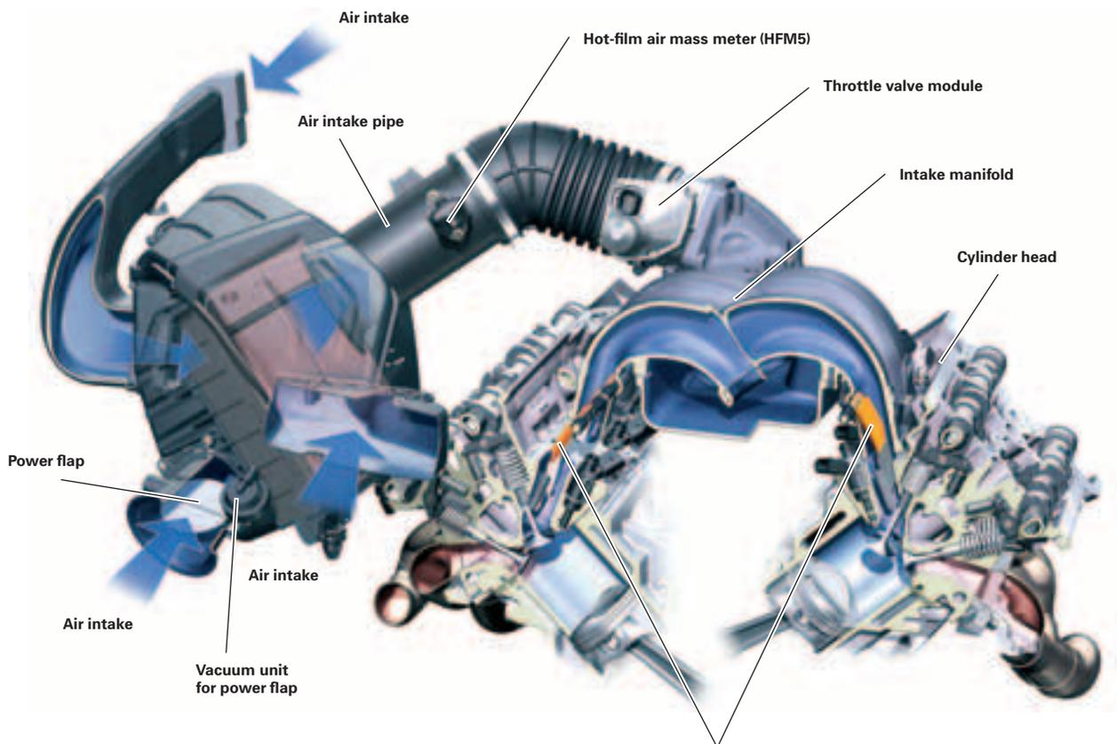
The RS4 engine does not have a variable inlet manifold.
