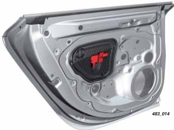
Left Access/Start Authorization Antenna R200
