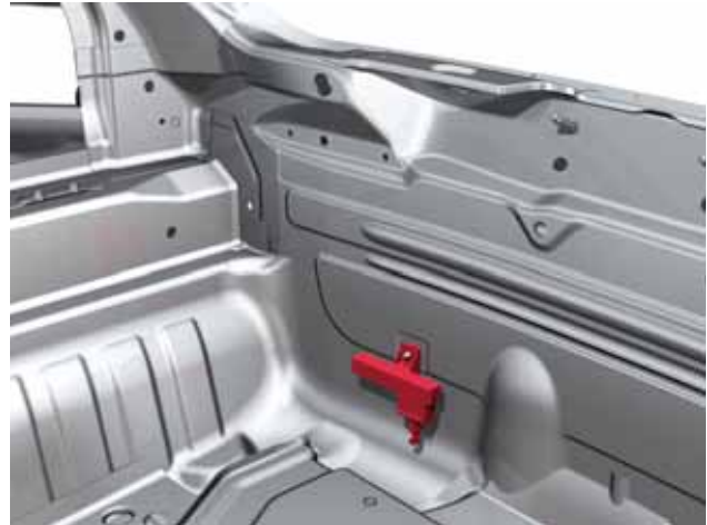
Access/Start Authorization Antenna in Luggage Compartment R137
