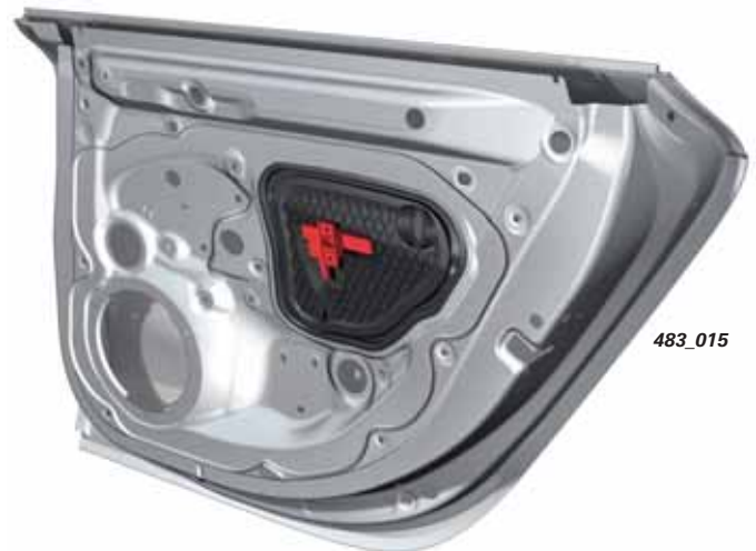
Left Access/Start Authorization Antenna R201
