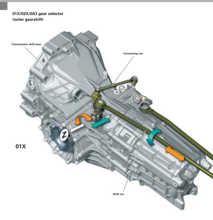
The fundamental design of the gear selector (outer gearshift) for the 01X/02X and 0A3 gearboxes is the same.
