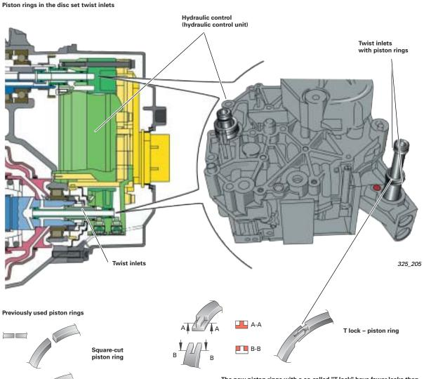
The new piston rings with a so-called "T lock" have fewer leaks than the previously used square- or diagonal-cut piston rings. The required oil feed quantity is lower, which in turn improves efficiency.
