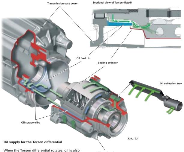
passed to the outer wall of the sealing cylinder. Most of this oil is scraped off by the oil scraper rib in the Torsen housing and is passed on to the slightly lower oil scraper rib of the transmission case cover. The oil then flows over the oil feed rib into the sealing cylinder and thus into the Torsen differential.
