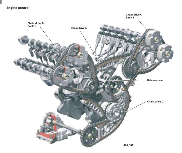
The chain drive is located at the power-output side of the engine. It is arranged over two levels. Four chains are installed in total.
