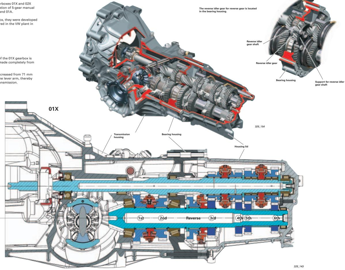
Axle base 75 mm The gear set is operated in the previously tried-and-trusted way for longitudinal Front gearboxes as a twin-shaft gearbox and for longitudinal quattro gearboxes using the original quattro hollow shaft.
