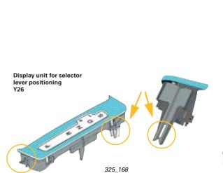
Once the shift sack has been unclipped, the display unit can also be unclipped.
