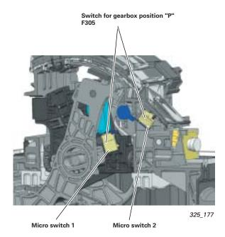
The information from selector lever position "P" supplies the two mechanical micro switches F305. They are connected in series and form one unit.
