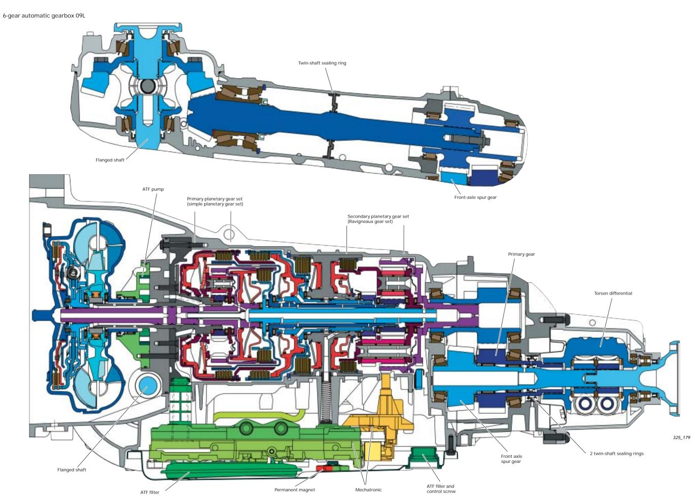
Gearbox cross-section 09L
