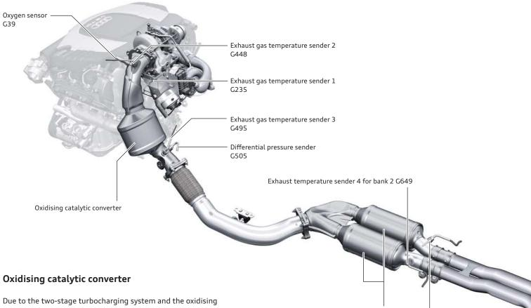
Due to the two-stage turbocharging system and the oxidising catalytic converter mounted on the engine bulkhead side, heating measures are necessary in order to ensure that the catalytic converter reaches its light-off temperature as quickly as possible after engine starting.
