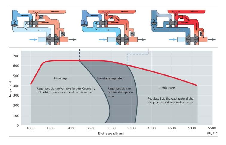
The described engine speed ranges in the various control modes shift under changing temperature and altitude conditions. The charge pressure control application factors this in when activating the actuators. When two-stage charging is employed, engine response is determined by the leak-tightness of the turbine changeover valve. Even the smallest of leaks can lead to high pressure losses in the high pressure turbine.
