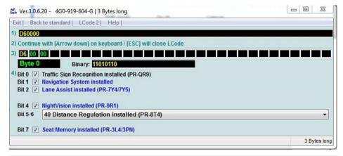
**Note:** You may need to change some adaptation channels associated with Traffic Sign Recognition system in order for HUD to be fully functional.
