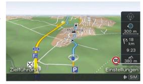
This procedure has the advantage that no additional components have to be fitted in the vehicle to implement the functionality. The map material that is used only has to contain prescribed speeds; these are then displayed when driving on the corresponding roads. However, the navigation data do not contain temporary prescribed speed limits, hence they cannot be displayed.
