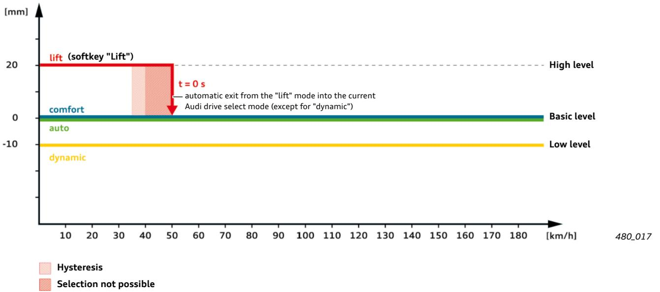
Control strategy of running gear / suspension 1BS (rough road version) without trailer operation
