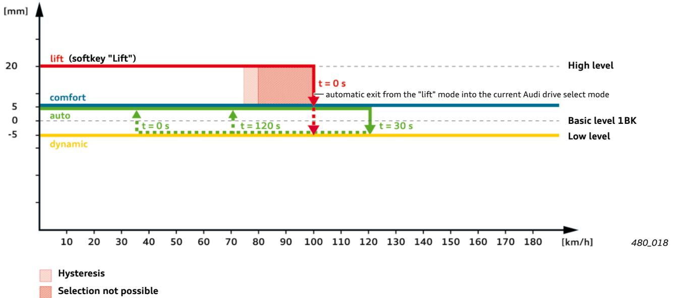
Control strategy for running gear / suspension 1BS with trailer operation
