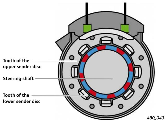
View from above in direction of the steering shaft (= axis of rotation)
