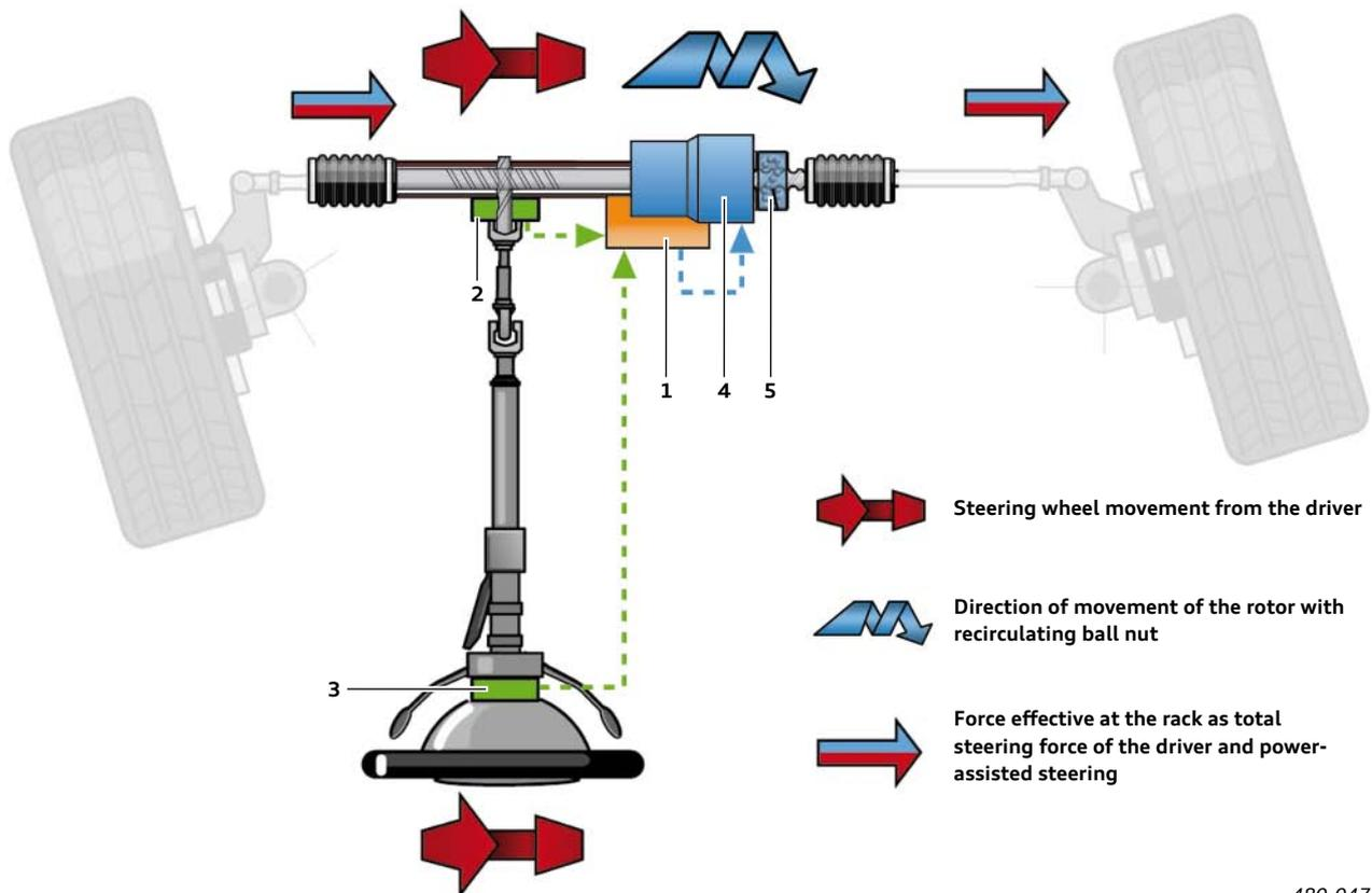
1. Control unit for electromechanical steering J500
