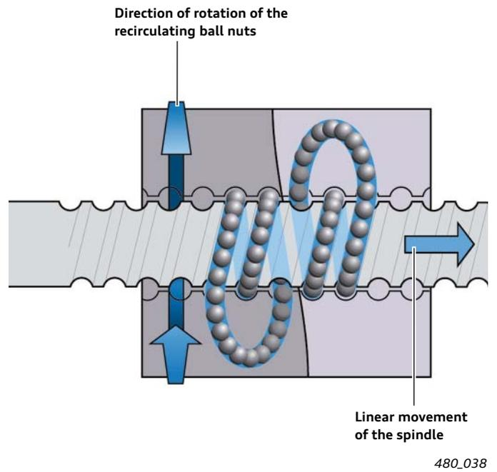
The recirculating ball nut is fixed in longitudinal direction. If it is turned, there is a linear movement of the spindle in the direction of the arrow.
