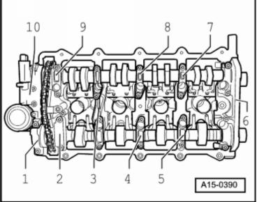
• The two camshaft markings must align with both arrows on bearing caps -arrows-.
