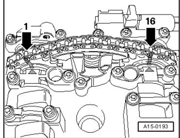
Secure camshaft adjuster using Bracket For Chain Adjustment -3366-.
