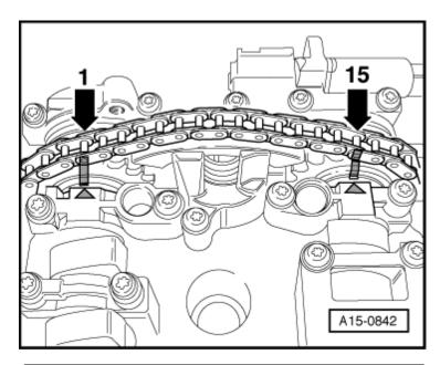
Secure camshaft adjuster using Bracket For Chain Adjustment -3366-.
