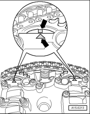
The distance between both -arrows- or colored markings consists of 15 rollers of the drive chain.
