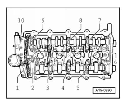
• The two camshaft markings must align with both arrows on bearing caps -arrows-.
