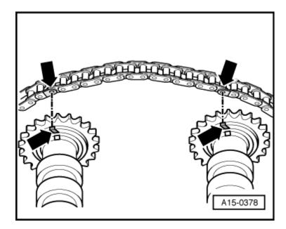
Distance between notches -A - and -B- at camshafts must be distance of 15 rollers at drive chain. Illustration shows where first and fifteenth drive chain rollers must be installed on chain gears.
