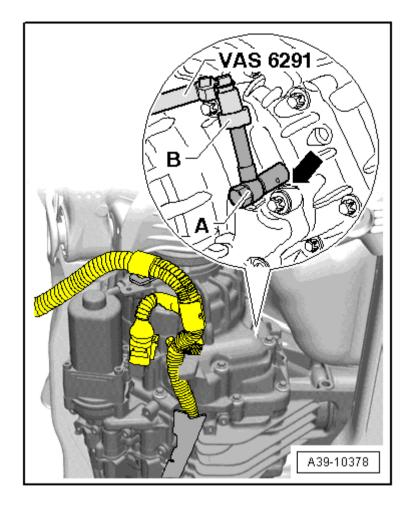
Screw in and tighten new gear oil inspection plug -arrow-. Tightening torque → Item
