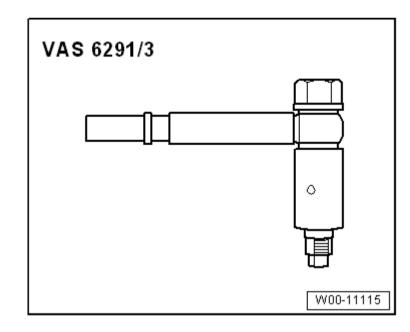
Depending on version, the spacer tube of the adapter for oil filling -VAS 6291/3- may make contact with a housing rib on the final drive.
