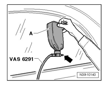
• The rear final drive is filled correctly when oil comes out between the adapter -A- and the rear final drive housing -arrow-.
