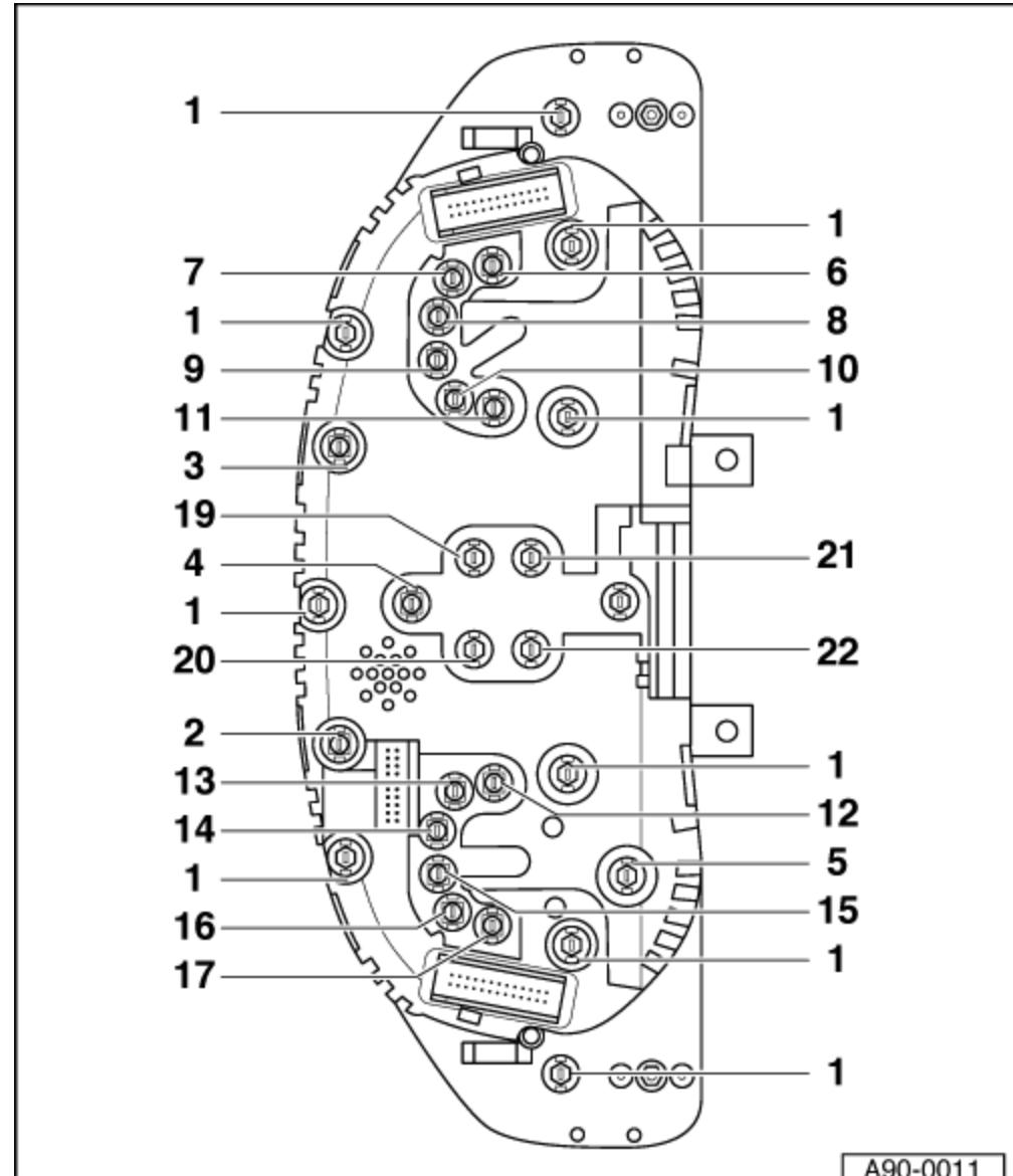
**8 - Traction control system warning lamp -K86- (ASR/TCS)**
