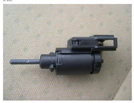
There have been numerous posts on the Vortex about failed brake light switches and a number of different
