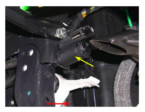
5. While holding the switch in place (DO NOT LET IT PUSH BACKWARDS - THIS IS CRITICAL), release the brake pedal and pull it back slowly as far as it will go (until it hits the stop), as indicated by the red arrow in the picture above. You should hear the plunger click as it compresses. This procedure sets the correct length for the switch plunger.
