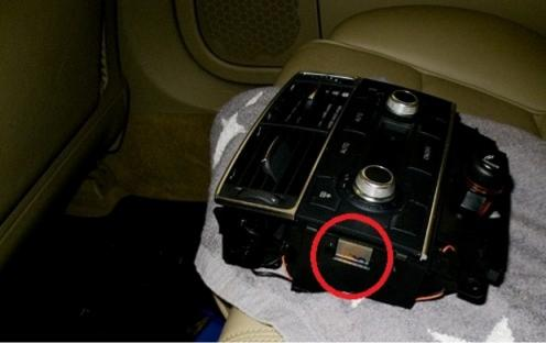
3. On to the instrument cluster trim. Push out the coin tray, grab the front and push it to the left so it comes off. You will remove the rest later.
