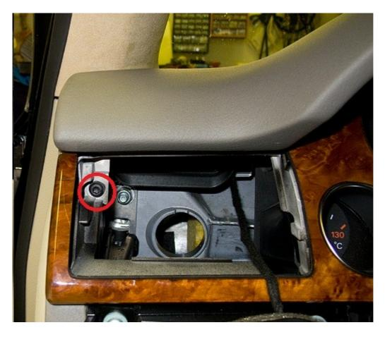
Remove the other vent as well and then you can wiggle out the trim. Put the new one in, refit the vents and screws.
