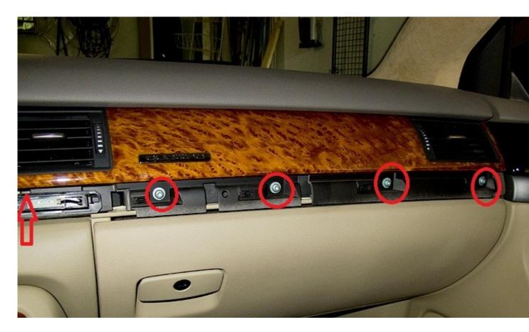
The coin tray needs to go as well so take a screwdriver or similar and insert it around the area of the red arrow in the above pic. Push down on it and the tray should come out.
