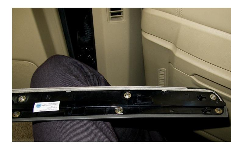
2. The rear console is of course a little different depending on your setup. In my case it's extermely simple. Just pry in the top corners and it will pop out. Remove and fit the new one.
