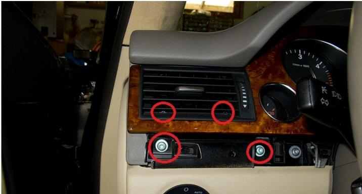
Before you can remove the trim you need to remove a hidden screw. So take some pointy tools and lift the tabs in the vent you see circled in the picture above. Once they are up far enough you can wiggle out the vent and behind it you will see a black allen screw that needs to be removed.
