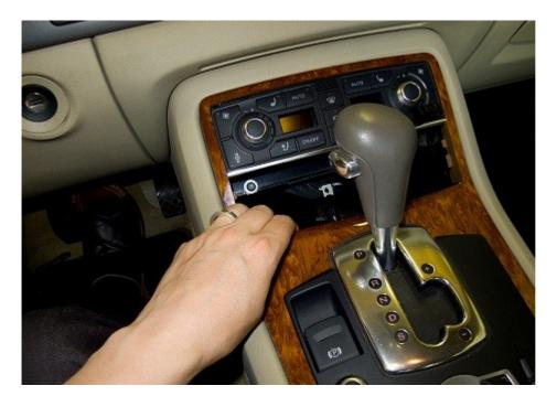
Remove the 4 T20 screws and transfer the control panel to the new trim. As you see in the pic I removed the cup holder bin as well but it was only because the rear alu trim on the new was in worse condition than the old one.
