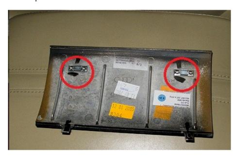
5. The one over the glove compartment: With the grey trim gone you see 5 T25 screws (leftmost missing in pic). The leftmost one holds a clip as well for the switch panel. Remove all 5.
