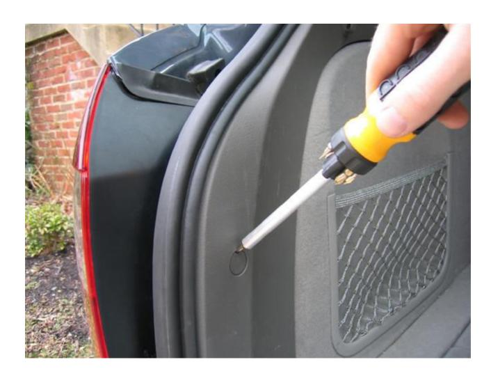
First I carefully opened the circular cover with a small flat head screw driver (it just pops out).
