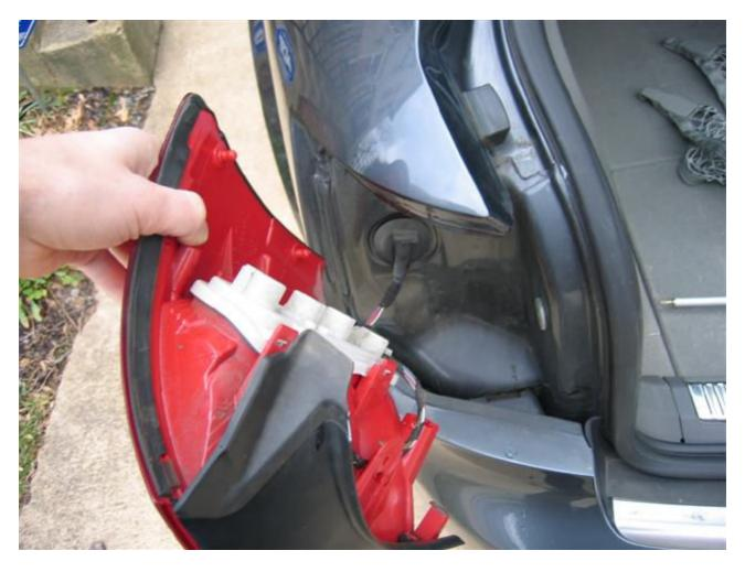
Once both plugs (top and bottom) were free of the body, the assembly was only connected by the wire.
