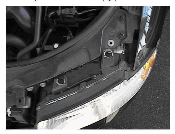
The third and fourth screw are a little harder to find, but shouldn't be too bad to get at. Just loosen these about 2 turns a piece and the entire assembly should become loose. Here's where to find them:
