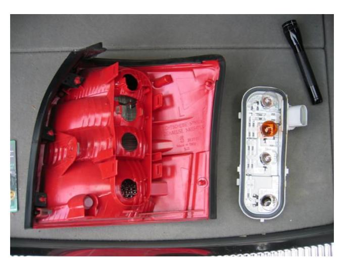
Finally I carefully separated the white piece from the assembly. The stop light bulb was the one at the bottom (it had two filaments). To remove it, I pressed down very gently and rotated it out counterclockwise.
