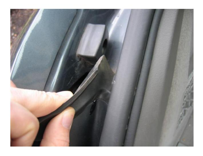
Once the assembly was free of the screw, I gently pulled back the rubber material so that it was free of that rubber block.
