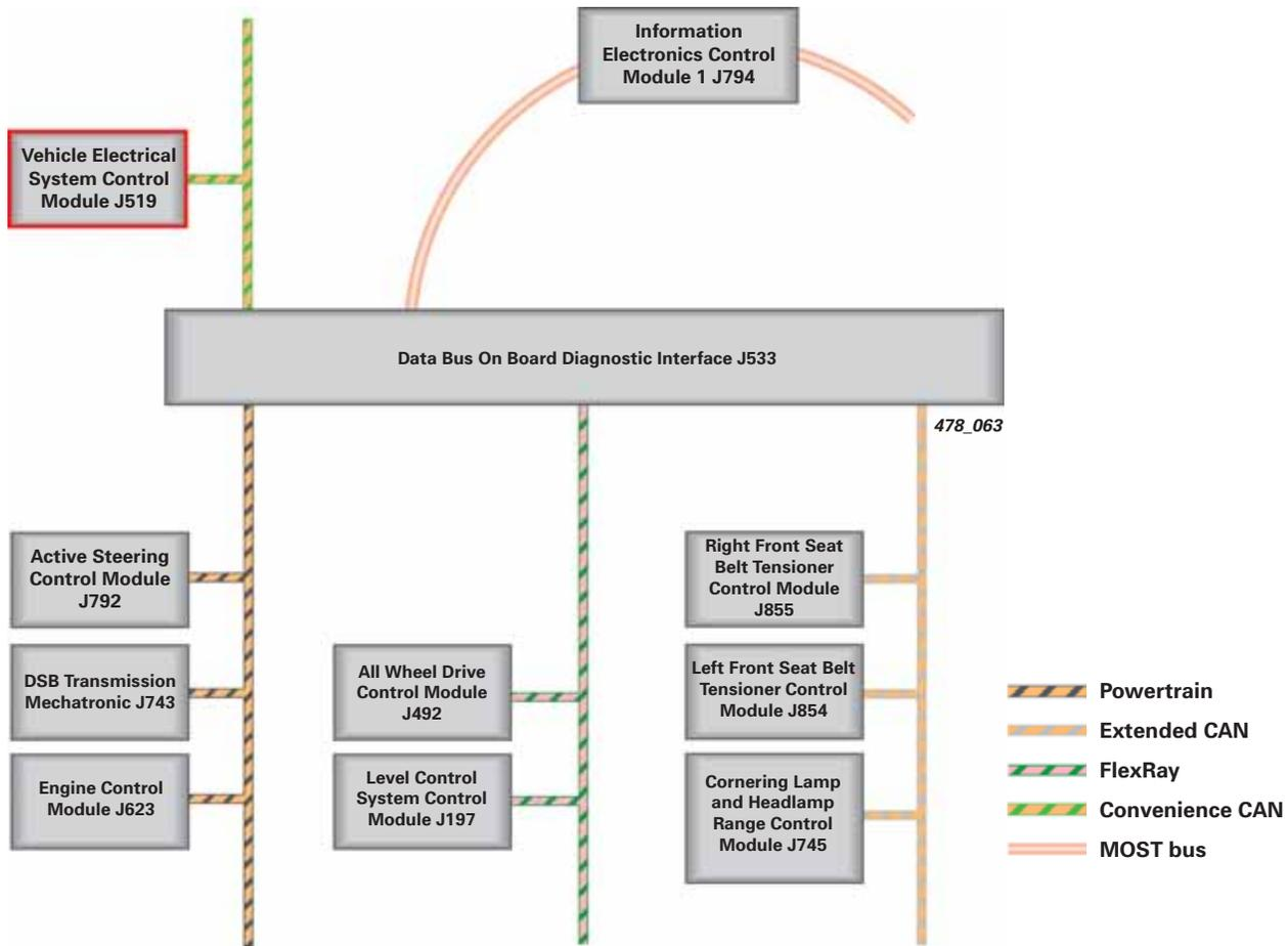
Vehicle Electrical System Control Module J519 performs the central function of Audi drive select. Information Electronics Control Module 1 J794 reads driver input information, transferring it to J519 via the MOST bus, Data Bus On Board Diagnostic Interface (Gateway) J533, and the Convenience CAN bus.
