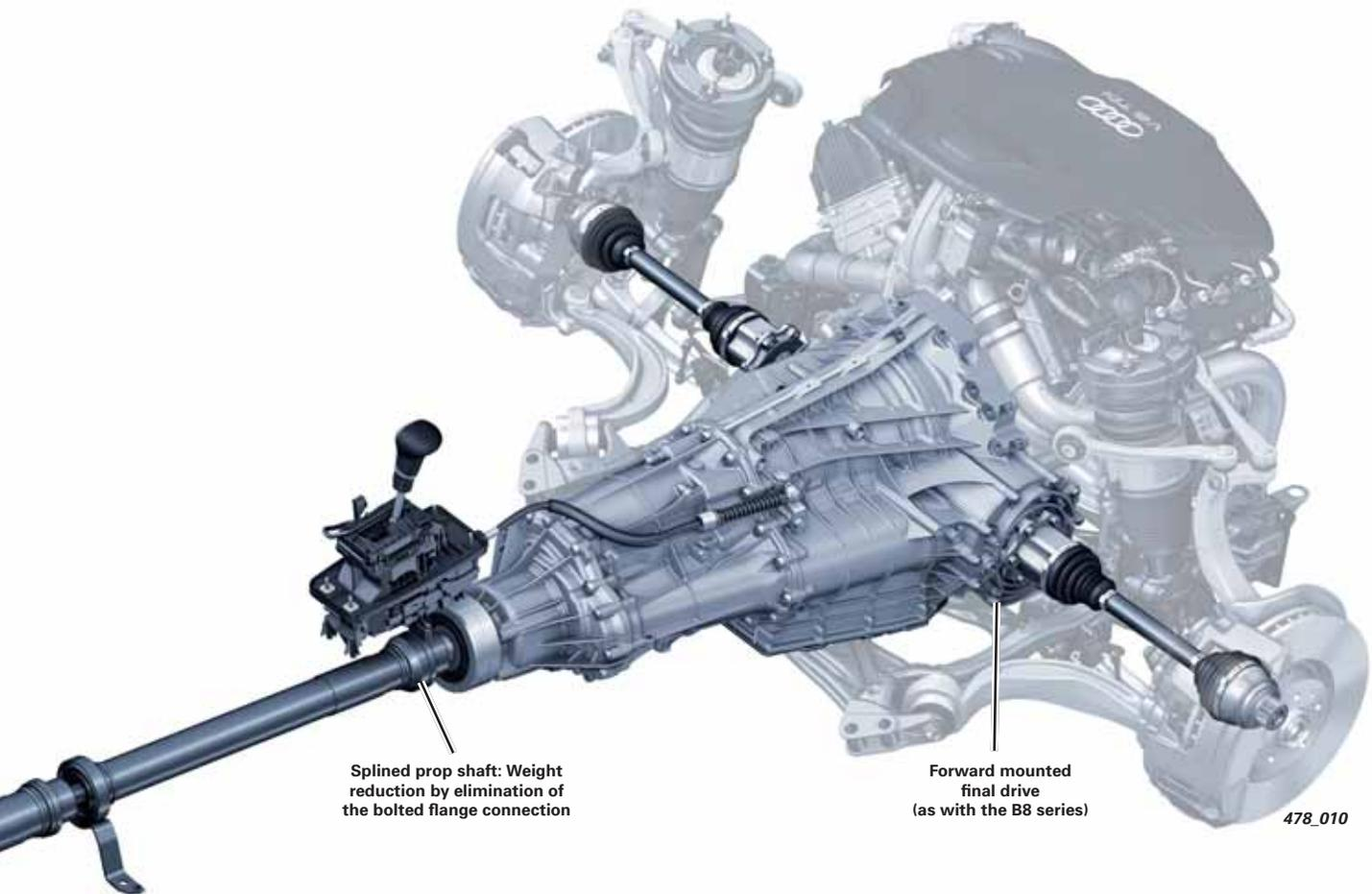
Splined prop shaft: Weight reduction by elimination of the bolted flange connection
