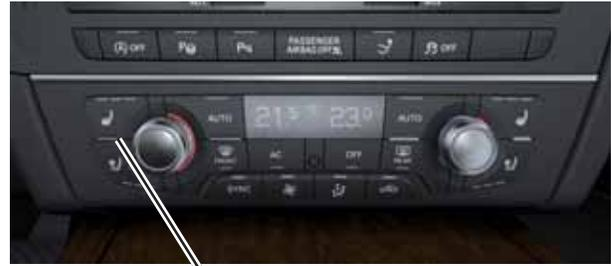
Seat heating/ventilation adjustment buttons
