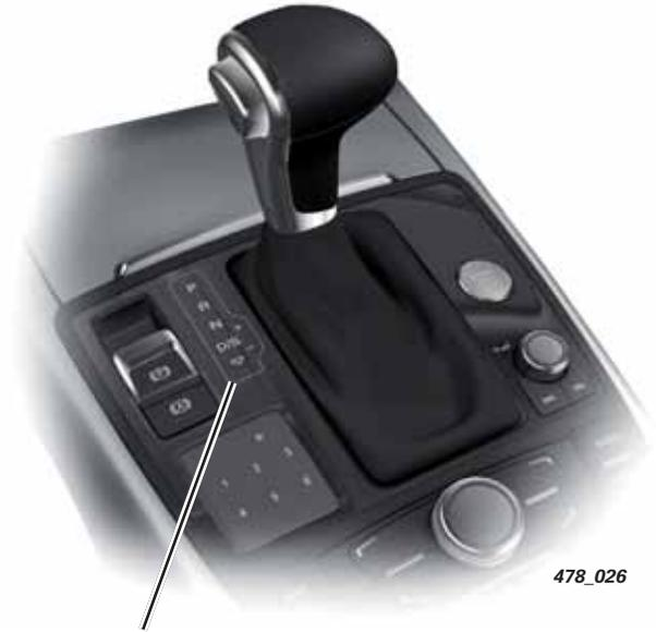
The shift pattern and indicator are integrated into the console trim frame. Selector Lever Transmission Range Position Display Unit Y26 is installed from below as a separate component.
