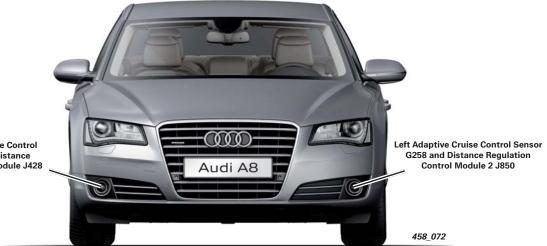
Right Adaptive Cruise Control Sensor G259 and Distance Regulation Control Module J428 Radar range has been increased compared to previous ACC systems. The measuring range begins approximately 1.6 ft (0.5 m) in front of the vehicle and extends to approximately 820 ft (250 m).
