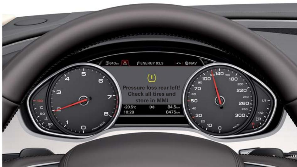
By evaluating the vibration characteristics of each wheel/tire, the new TPMS system is capable of determining and indicating which tire is experiencing pressure loss.
