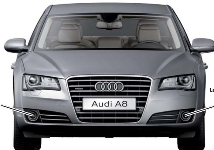
Left Adaptive Cruise Control Sensor G258 and Distance Regulation Control Module 2 J850
