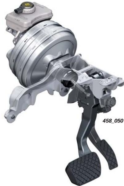
The master brake cylinder, brake fluid reservoir, and pedal assembly are adopted from the current Audi A4.
